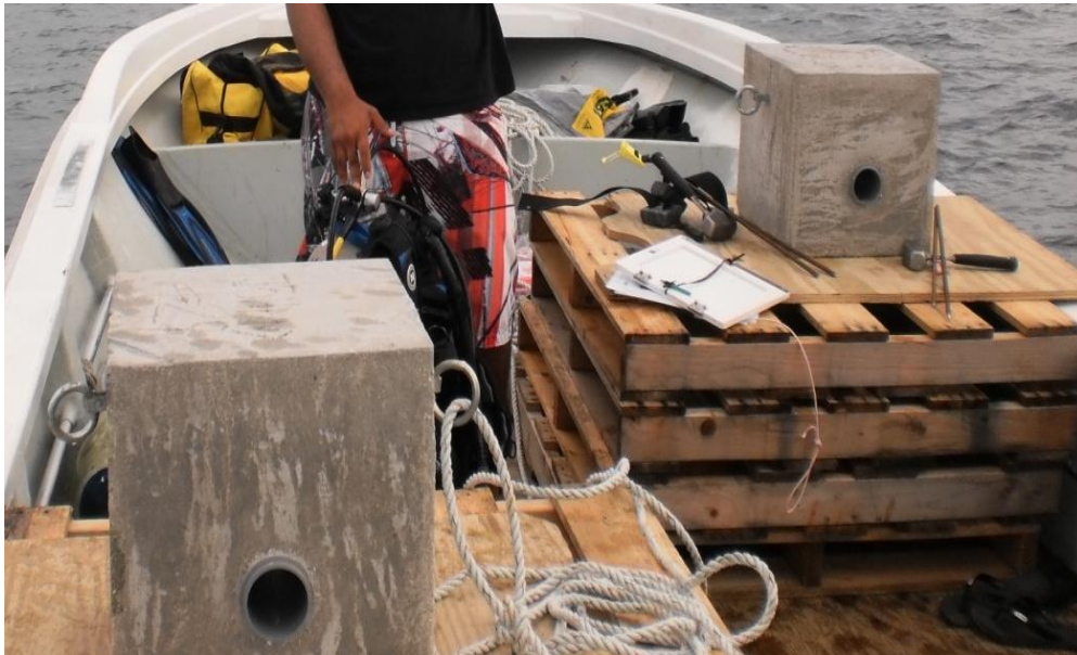
Figure 4 Concrete housings for the temperature logger being readied for deployment at Majuro Atoll, 2011.
