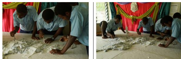
Once dry and secure, the model is covered with a thin paper, pasted using acrylic white or translucent gel medium. This paper smoothes out the contour layers and helps with terrain continuity.
