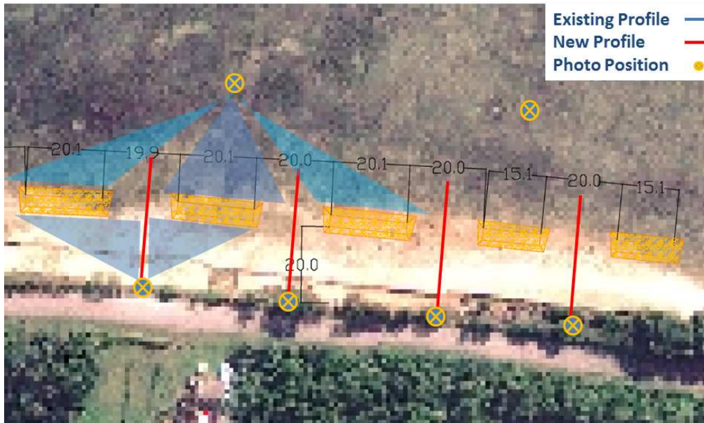
Figure 2.6. Camera shot angles from the landward end of each beach profile and from offshore looking landward towards each detached breakwater.
