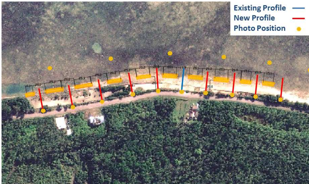
Figure 2.5. Beach profile and camera/photograph locations eastern Manuka.
