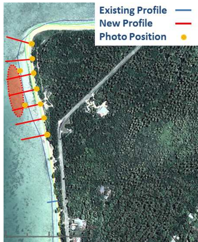
Figure 2.7. Beach profile and camera/photograph locations at Whitehouse Point.
