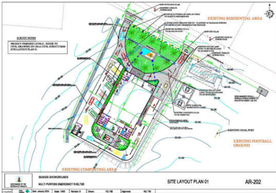
Figure 3.1: Seaside site layout plan showing replacement of the existing basketball court and the replacement of the existing small market stall (food stall):
